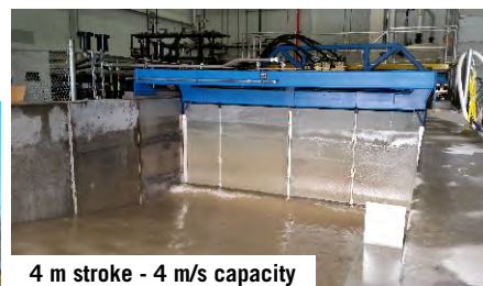
4 m stroke - 4 m/s capacity
